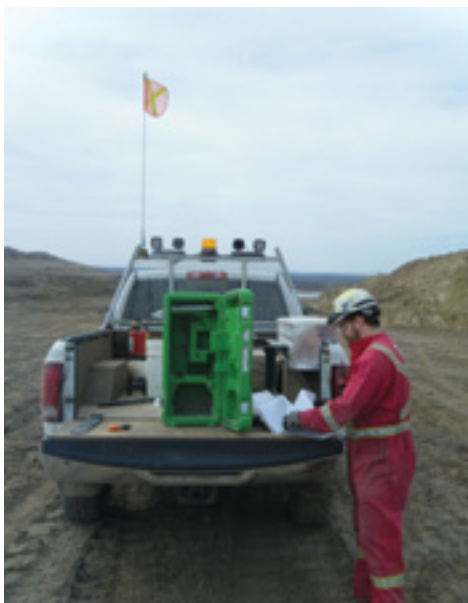
A Norwest construction monitoring technologist collects and records compaction and other construction data in the field.
